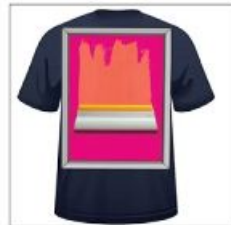
Step Seven Ink is applied to open areas of screen with a squeegee. Repeat for each color (including base as needed).
