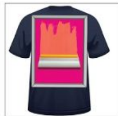
Step Seven Ink is applied to open areas of screen with a squeegee. Repeat for each color (including base as needed).
